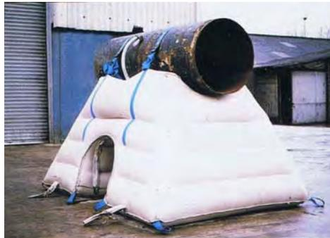
Pipe Support Block Test
