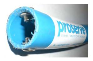
1" outside diameter plastic water pipe with 2 stainless steel riveted electrodes to maintain accurate measurement.
