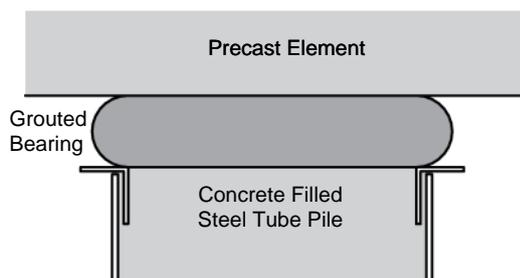
Figure 8—Pile Bearing
