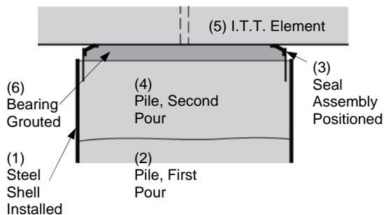
Figure 26 – Pile Bearing Detail
