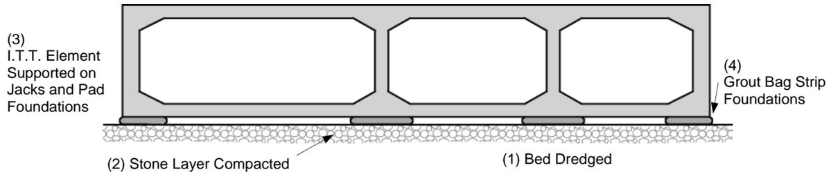
Figure 24—Construction Sequence
