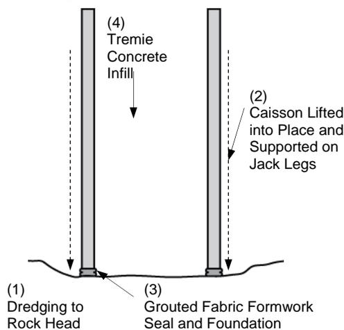
Figure 16 – Construction Sequence
