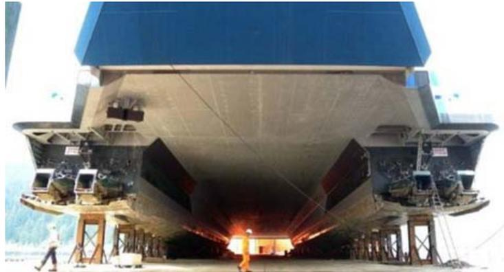
Figure 3: Fast Ferry Hull and Jets
