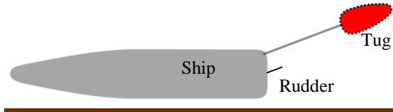
Figure 5. Berthing with a Single Stern Tug
