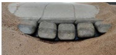
Figure 43. Test 1, Deployed, Tight Geotextile
