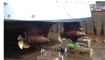
Figure 2. Azipods in dry dock
